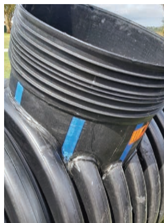
1200mm pipe with a 630mm riser
