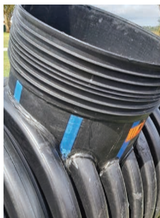
1200mm pipe with a 630mm riser
