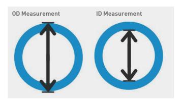
**Nominal bore** (NB) is never an exact measurement. By definition, 'nominal' means in-name-only, or a referenced name. The problem with nominal bore measurements is often the part number uses nominal bore not the actual size you are looking for. The tables below further define these terms with regards to specific stock.
